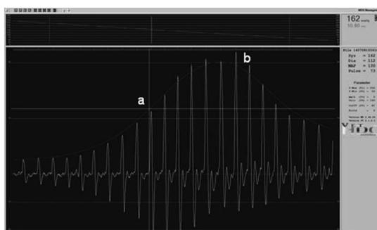
**Figure 2.** An example of an excellent trace, displaying linear deflation (upper section) and a complete bell-shaped curve devoid of strong movement artefacts in the key period (lower section). The key period is between systolic (a) and diastolic measurements (b).
