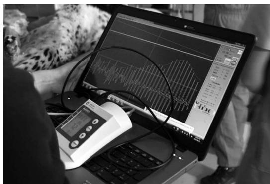
**Figure 1.** The Vet HDO MD Equine, which has a numerical display, is connected to a laptop that allows visualization of the pressure waveform.
